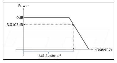
Figure 3: An amplifier's bandwidth is determined by its -3dB point
