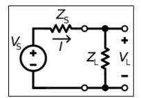
Figure 2: Source & load impedance
