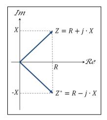
Figure 1: Source & load impedance are complex-conjugates.
