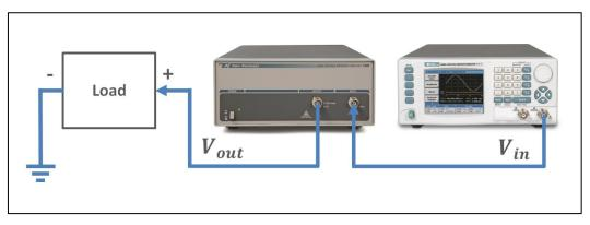
Figure 7: Tabor's Signal source + amplifier driving a load
