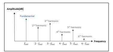
Figure 6: Spectral view of a distorted non-ideal tone
