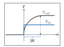
Figure 4: An amplifier's non-linear rise time, in response to a step voltage input
