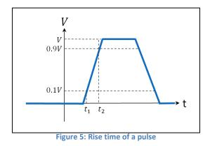
Slew rate is usually specified with information on the setup it was measured with, including the impedance of the load used.
