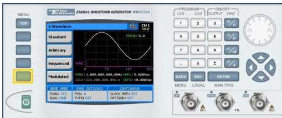
4. Press the **Modulation Type** menu button. A list of modulation types appears on the screen. By default, the modulation type is set to "OFF".
