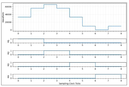
Figure 8.2 P2582M Model 8 Waveform Points and 4 Marker Points
