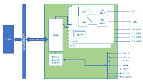
Figure 5.2 Proteus Block Diagram
