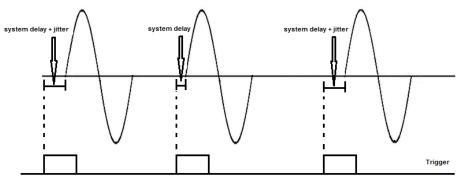
Figure 9.4 Trigger Jitter and System Delay
