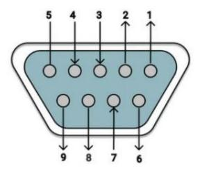
Figure 12.1 D-Sub 9-Pin Female Pin Numbering
