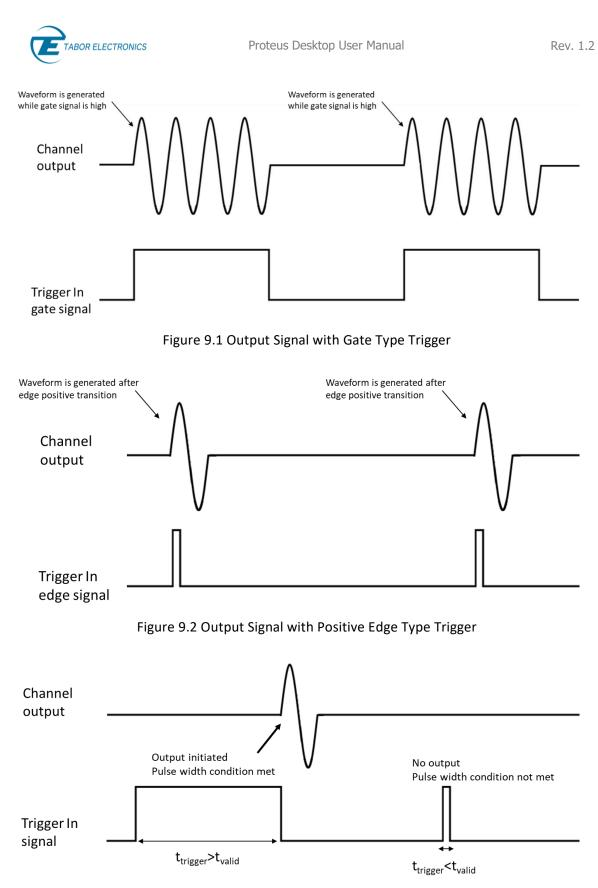
Figure 9.3 Outputs Behavior with Pulse Detect Width Set to Time  $t_{valid}$
