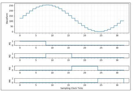
Figure 8.1 9 GS/s Model - 32 Waveform Points and 4 Marker Points
