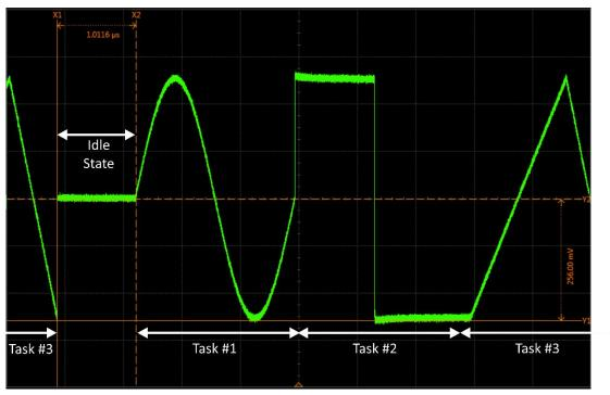
Figure 7.3 DC Level Idle State Associated to Task #1
